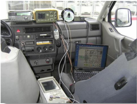
Tel Aviv, Israel – Mobile Installation, visible DFP-1000B, KVH-1000 Digital Compass, Garmin GPS, AOR5000 Radio Receiver, Spectrum Analyzer and Laptop running HuntMaster
