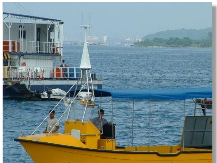
Singapore – Singapore's Navy rapid interception vessels equipped with DF Triangulation capabilities
